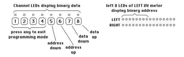
The left 8 LEDs of the left channel VU meter display a binary memory address--LED off=0, LED on =1. When you first enter programming mode, the address will be 27 (00011011 on the VU display). Press the channel 5 button to decrement the address or the channel 6 button to increment the address. Silence sensor related address are shown in the table below.
