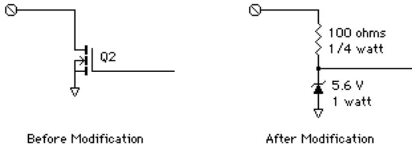
After Q2 is removed, the new parts can be installed vertically using the same holes in the PC board. The zener diode helps to protect against voltage transients and the 100 ohm resistor acts to limit current. This circuit will drive most solid-state relays directly without the need of an external voltage source.
