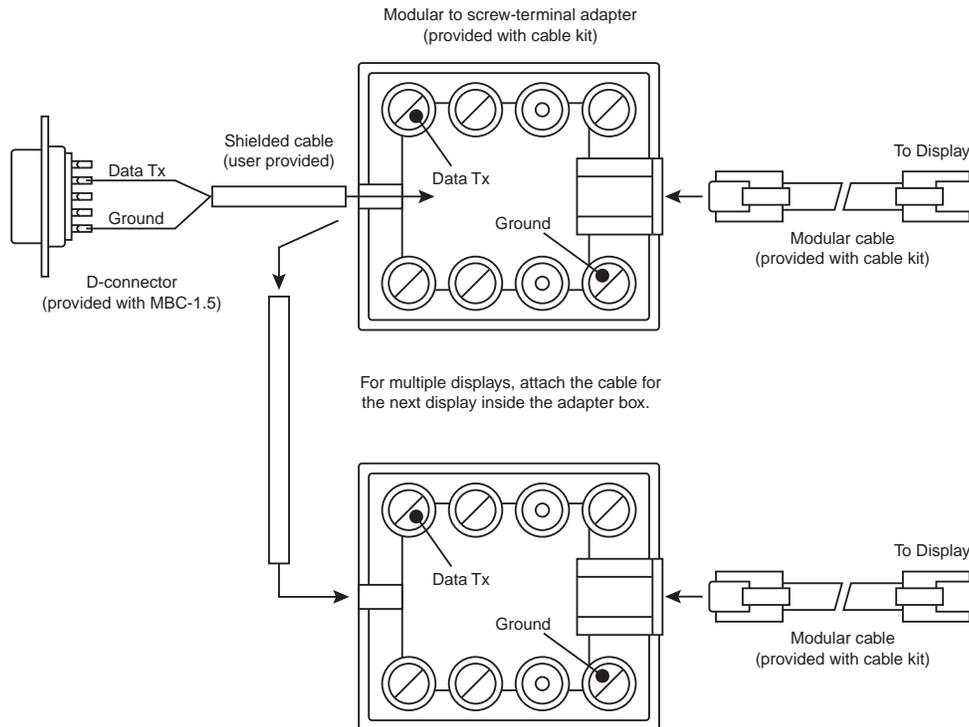
Multiple displays are connected between the adapter boxes. Each display connects to the adapter of the previous.
