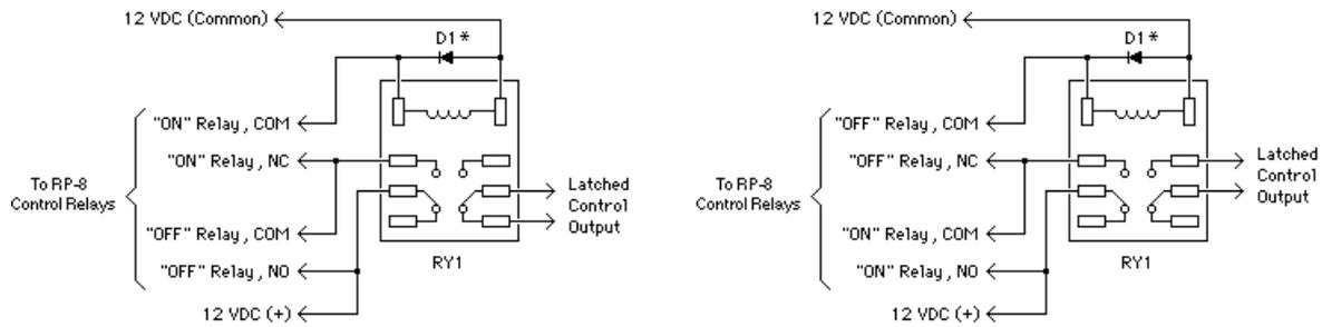
Note: This circuit "powers up" with the latched output "ON."
