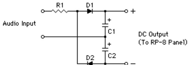
R1 is 470 ohms (Radio Shack 271-1317), D1 and D2 are 1N4001 (Radio Shack 276-1101), and C1 and C2 are 470  $\mu$ F/16V (Radio Shack 272-957). Any audio level of -6 dBv or greater will maintain at least 0.5 volts DC at the output. This covers most "line level" audio sources.
