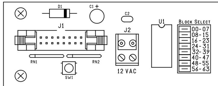
Place the jumper on the pair of pins next to the appropriate range of channel numbers for each SIP-8. Ensure that each RP-8 and SIP-8 in a system is set to a different block (range of channels). Blocks are usually used continuously from channel 00 up but a block of channels may be skipped if necessary.
