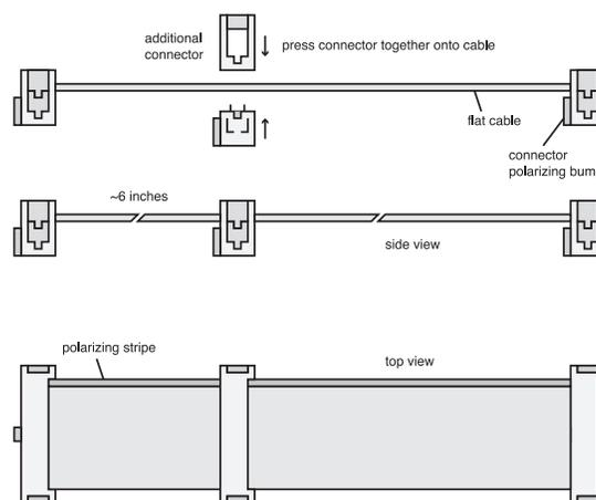
Ensure that the connector is aligned directly across the cable. If the connector is at an angle, the metal teeth on the connector may penetrate the cable insulation at the wrong points and short the conductors or miss them entirely.
