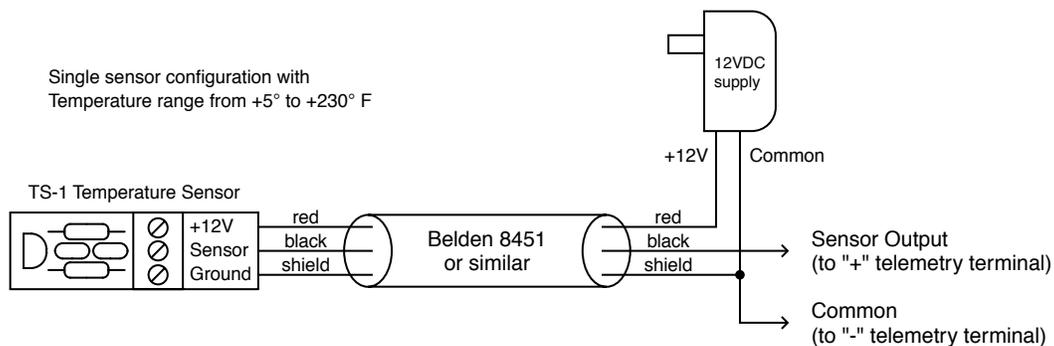
Figure 1; Single sensor with temperature range +5° to +230° F
