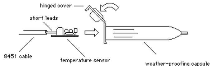
*Figure 5; Temperature sensor in weather proofing capsule*
