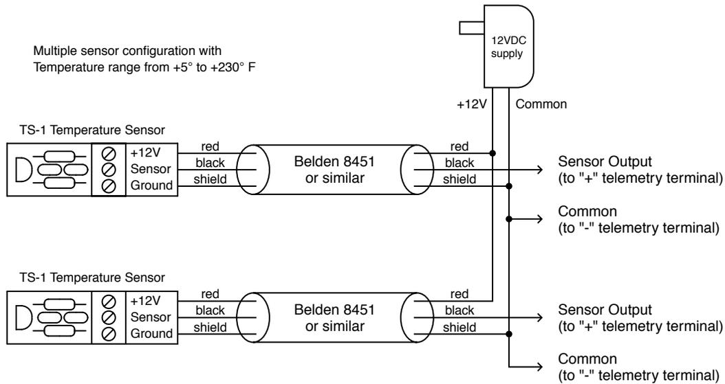
Figure 2; Multiple sensors with temperature range +5° to +230° F
