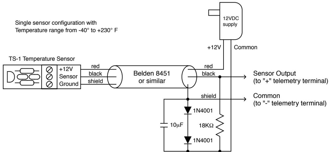
Figure 3; Single sensor with temperature range -40° to +230° F
