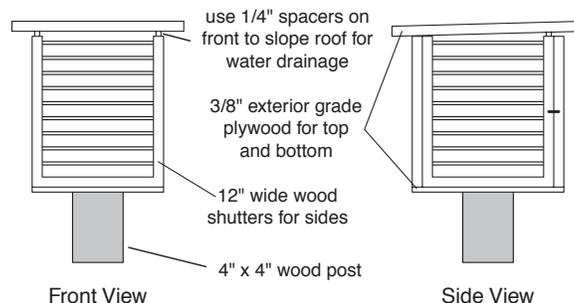
Figure 3.4; Standard enclosure for temperature sensor
