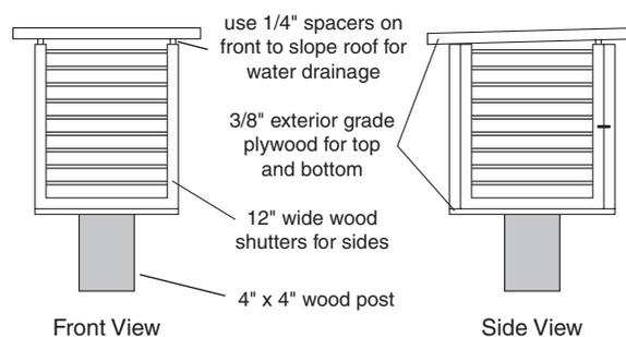
Figure 3.4; Standard enclosure for temperature sensor
