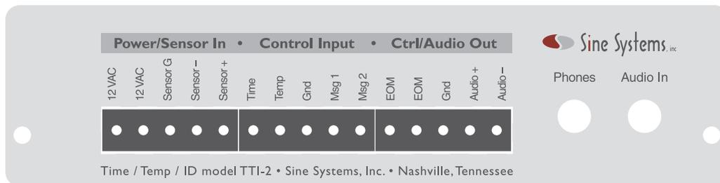
Figure 3.1; TTI-2 Rear Panel Connections
