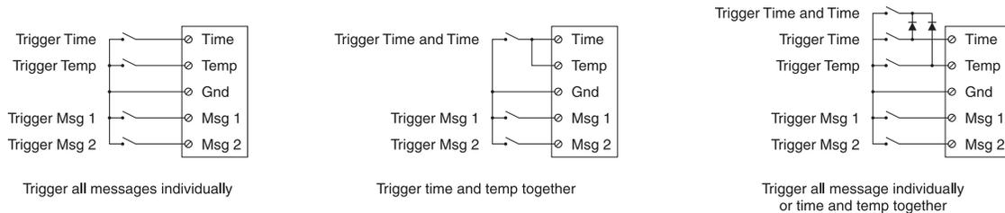
Figure 3.2; Example external trigger wiring
