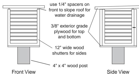
Figure 5.2; Standard enclosure for temperature sensor
